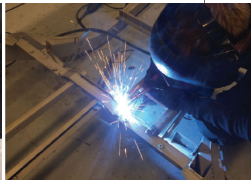
Welding the battery carrier
