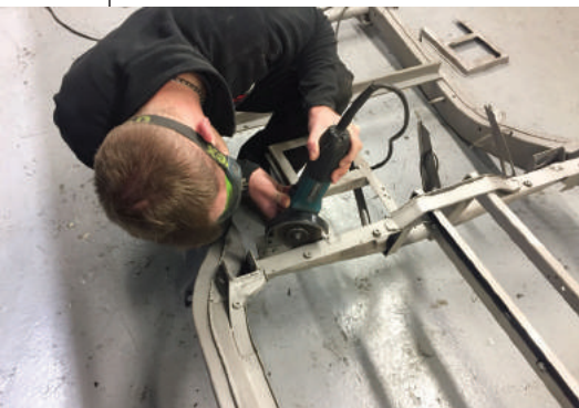
Grinding out the unwanted battery carrier
