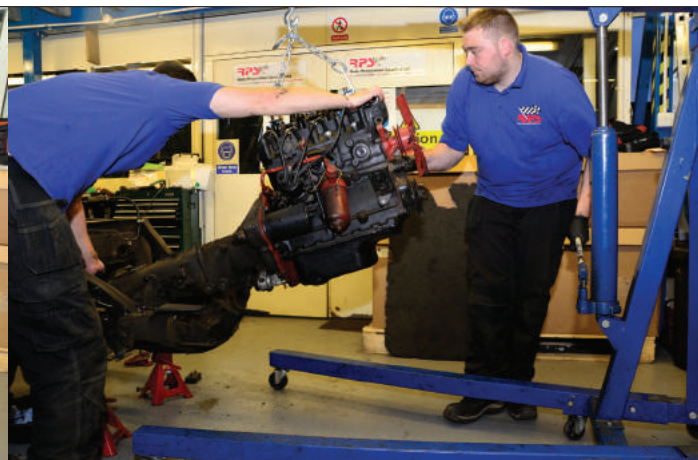
Engine being guided away from the chassis
